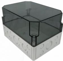
An **IP66 Rated, Grey (RAL7035) Enclosure** designed for use with the Hochiki range of DIN Modules. Supplied with a transparent black lid as standard. The unit is supplied with a DIN Rail section (plus fixings) and will accept up to six Hochiki DIN Rail Modules, side-by-side.
