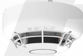
An **Intelligent Multi-Heat Sensor** incorporating a variable Fixed Temperature heat element and Rate Of Rise heat element, both controlled from the Control Panel allowing either thermal element or both elements simultaneously to be active in making the fire decision.
