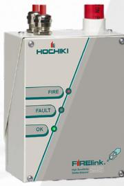
A **Single Pipe Air Sampling Detector** designed to provide very high sensitivity smoke detection. The unit will automatically setup for easy installation and is also designed to fit into a Docking Station which accepts all sampling pipes and cables leaving the detector to be fitted during the final commissioning phase.
