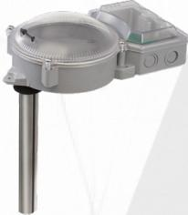
A **Duct Probe Housing** allowing a standard photoelectric smoke detection device, either a conventional detector or an analogue sensor, to be mounted on the outside of an air duct for the purpose of monitoring the air within the duct.
