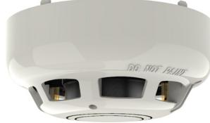
An **Intelligent Multi Sensor** incorporating a thermal element and a High Performance photoelectric smoke chamber. Has three modes controlled from the Control Panel, allowing either the optical or thermal element or both to be active in making the fire decision.
