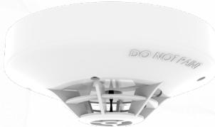
An **Intelligent IP67 Rated Waterproof Multi-Heat Sensor** which can be used externally and is supplied with its own fixing base which is used to fix the sensor. Flying leads from the sensor connect directly to the loop via waterproof connectors.
