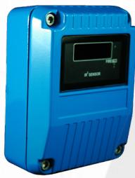
A **Conventional IR<sup>3</sup> Infrared Flame Detector** designed to respond to low-frequency (1 to 15Hz) flickering IR radiation emitted from flames during combustion, the unit can discriminate between flames and spurious sources of radiation such as sunlight. An I.S. version and an explosion-proof version are also available.
