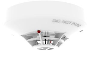
A **Conventional 90°C Fixed Temperature Heat Detector** using a thermistor and linearising circuit to provide an accurate linear response. A third terminal provides integral remote indicator output.
