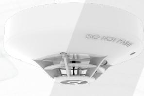
A **Conventional Rate of Rise Heat Detector**, Rate of Rise with 90°C temperature element. The thermistor and linearising circuit provide an accurate linear response Heat Detector. A third terminal provides integral remote indicator output.
