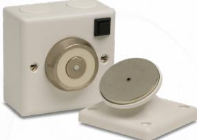
An **Electromagnetic Door Holder** designed to hold open fire doors and is ideally suited for hospitals, schools and other public buildings. In a fire situation the doors can be released automatically via a connection to the fire alarm system or manually by activating the release button.
