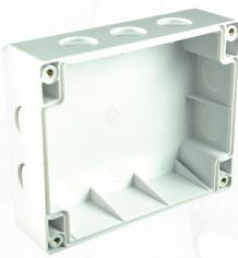
The **Module Backbox** is designed for installations where the CHQ Range of Modules - CHQ-DIM(SCI), CHQ-SZM(SCI), CHQ-DZM(SCI), CHQ-DSC(SCI), CHQ-MRC(SCI), CHQ-DRC(SCI) & CHQ-PCM require mounting within a glanded enclosure. The unit features ten knock-outs suitable for cable glands (not supplied) and accepts the CHQ Modules directly as a lid.
