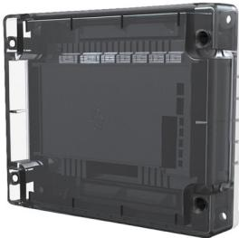
An **Analogue Dual Zone Monitor** which is fully compatible with Hochiki's ESP analogue addressable protocol and I.S. equipment. The module will allow connection of up to 40 Hochiki I.S. conventional detectors (20 per zone) through a Galvanic isolator, which are fully monitored for open and short circuit. The unit also features an integral short-circuit isolator.
