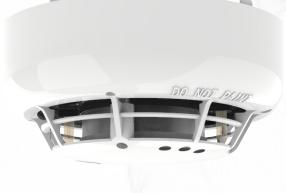
**Addressable Multi Sensor with CO detection**, an addressable loop-powered multi-sensor, with smoke, heat and CO sensing elements. The unit offers 24 different modes of operation\* and seamlessly matches the other sensors in the ESP range. The CO sensing element can be used to detect smoke as well as life-threatening CO levels (acting as a CO alarm).
