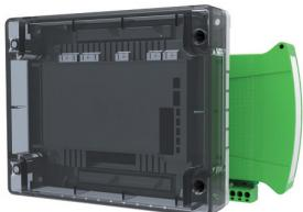
An **Intelligent Dual Sounder Controller** which has been designed to provide two sounders outputs (that can be driven separately) with full fault monitoring. The monitored input can be used for local power supply fault monitoring or as a general-purpose input. Feature an integral short-circuit isolator.
