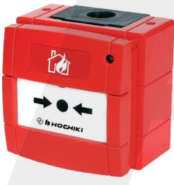
A **Marine Approved Intelligent Weatherproof Manual Call Point** fully compatible with Hochiki's ESP analogue addressable protocol and featuring an integral short-circuit isolator (SCI). Features a bi-coloured LED to indicate either fire (red) or short-circuit (amber). Also features plug-in wiring terminals for easy installation.
