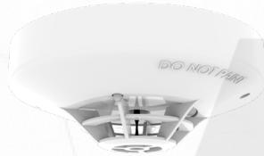
A **Conventional Rate of Rise Heat Detector** incorporating a 60°C fixed temperature element. The thermistor and linearising circuit provide an accurate linear response Heat Detector. A third terminal provides integral remote indicator output.
