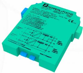
This **Isolated Barrier** is used for intrinsic safety applications. The device transfers DC signals of fire alarms and smoke alarms from the hazardous area to the non-hazardous area. The device can also be used to control I/P converters, valves, indicators, and audible alarms.
