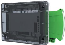
An **Intelligent Single Zone Monitor** designed to allow up to 6 conventional detectors or 1 SPC-ET to be interfaced to Hochiki's ESP analogue addressable system. Feature an integral short-circuit isolator.
