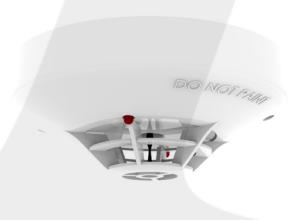
A **Conventional 60°C Fixed Temperature Heat Detector** using a thermistor and linearising circuit to provide an accurate linear response Heat Detector. A third terminal provides integral remote indicator output.
