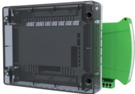
An **Intelligent Mains Relay Controller** providing a single mains rated relay output for the control of such devices as dampers, extractors or plant and equipment shut-down. The monitored input can be used for local power supply fault monitoring or as a general-purpose input. Feature an integral short-circuit isolator.
