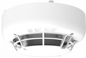
An **Intelligent Photoelectric Smoke Sensor** incorporating Hochiki's unique High Performance Chamber which allows the sensor threshold level to be increased, thereby improving the signal to noise ratio and reducing susceptibility to false alarms.
