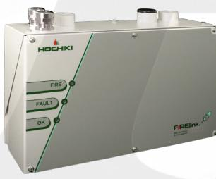
A **Two Pipe Air Sampling Detector** designed to provide very high sensitivity smoke detection. The unit will automatically setup for easy installation and is also designed to fit into a Docking Station which accepts all sampling pipes and cables leaving the detector to be fitted during the final commissioning phase.
