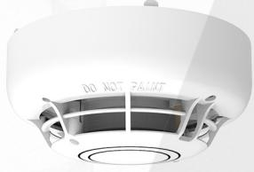
An **Intelligent Multi Sensor** incorporating a thermal element and a High Performance photoelectric smoke chamber. Has three modes controlled from the Control Panel, allowing either the optical or thermal element or both to be active in making the fire decision.
