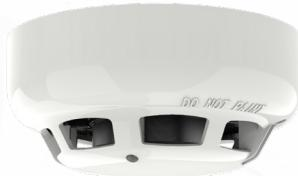
An **Intelligent Photoelectric Smoke Sensor** incorporating Hochiki's unique High Performance Chamber which allows the sensor threshold level to be increased, thereby improving the signal to noise ratio and reducing susceptibility to false alarms.
