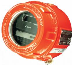
A **Conventional Explosion-Proof Infrared Flame Detector** designed to respond to low-frequency (1 to 15Hz) flickering IR radiation emitted from flames during combustion, the unit can discriminate between flames and spurious sources of radiation such as sunlight.
