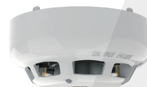
An **Intelligent Multi-Heat Sensor** incorporating a variable Fixed Temperature heat element and Rate Of Rise heat element, both controlled from the Control Panel allowing either thermal element or both elements simultaneously to be active in making the fire decision.
