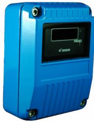
An **Intrinsically Safe Conventional Infrared Flame Detector** designed to respond to low-frequency (1 to 15Hz) flickering IR radiation emitted from flames during combustion, the unit can discriminate between flames and spurious sources of radiation such as sunlight.
