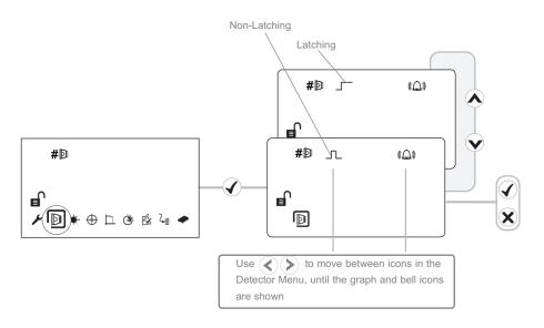
To clear a latched fire, apply 5-40V to the External Reset terminal, enter the passcode, or power cycle for 20s
